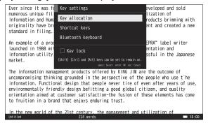
2 Select [Key allocation] with the ∧ / ∨ keys, and press the enter key
